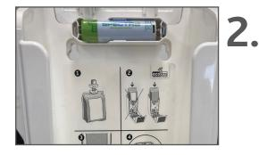
A battery is located within the dispenser (on earlier models the battery can be found at the back of the dispenser). The battery can be removed and charged directly via the usb micro port.
